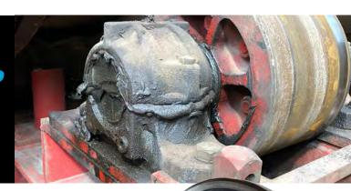
But, how you choose to grease your bearings is an important decision. It's estimated that 55% of mounted bearings fail because of lubrication problems and another 25% fail due to contamination issues. Grease purge from bearings also create safety hazards such as slips and falls, increases the risk of fires and can be considered a hazardous material. The conventional daily greasing of bearings is also a major expense, costing as much as 5X the initial cost of the bearing!
